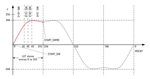
Figure 13.1 LUT programming example
