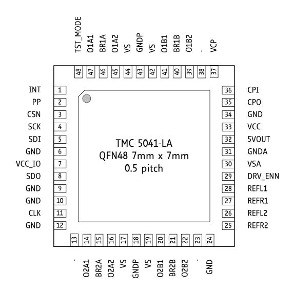
Figure 2.1 TMC5041 pin assignments.
