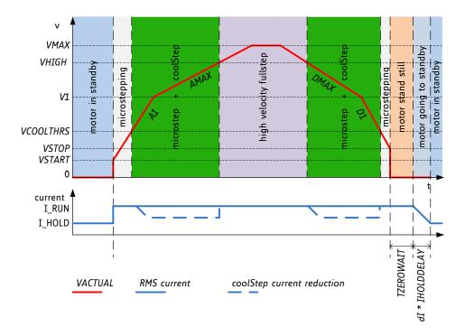
Figure 10.3 Ramp generator velocity dependent motor control
