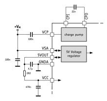
Figure 3.4 RC-Filter on VCC for reduced ripple
