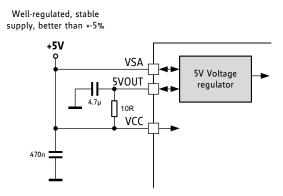
Figure 3.3 Using an external 5V supply to bypass internal regulator
