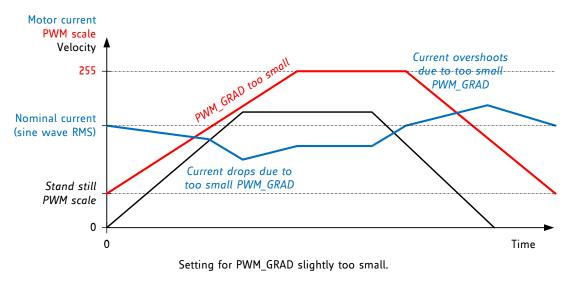
Figure 7.4 Good and too small setting for PWM\_GRAD
