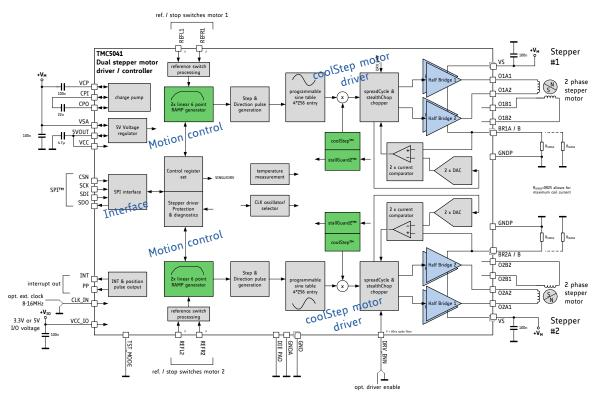
Figure 1.1 Basic application and block diagram
