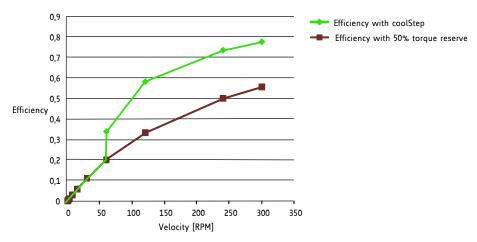
Figure 1.2 Energy efficiency with CoolStep (example)
