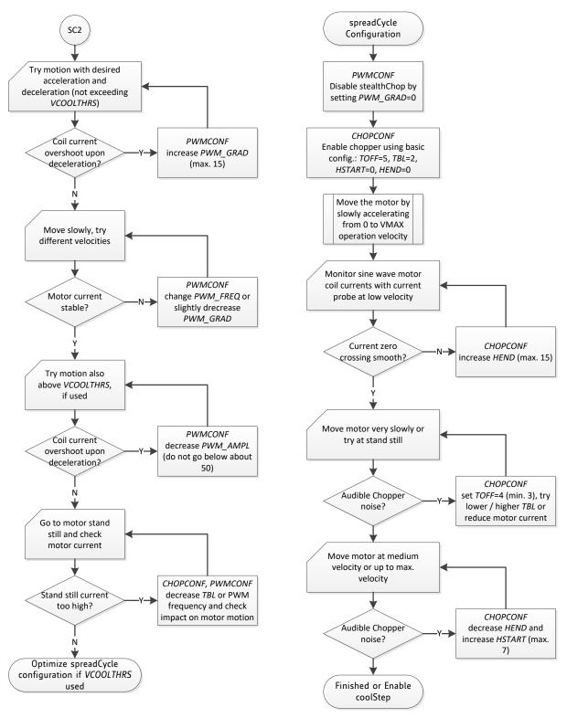
Figure 14.2 Tuning StealthChop and SpreadCycle
