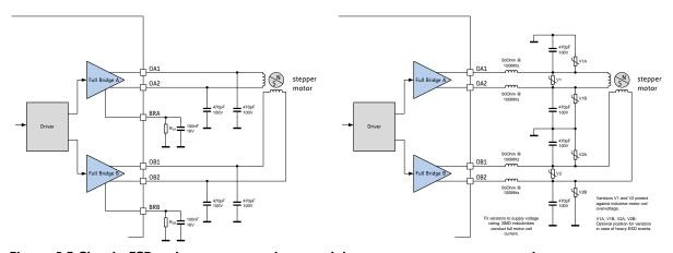
Figure 3.5 Simple ESD enhancement and more elaborate motor output protection
