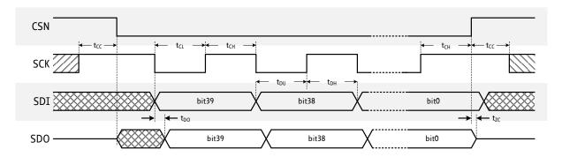
Figure 4.1 SPI timing
