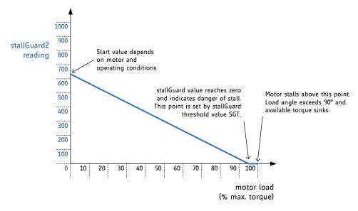
Figure 11.1 Function principle of StallGuard2
