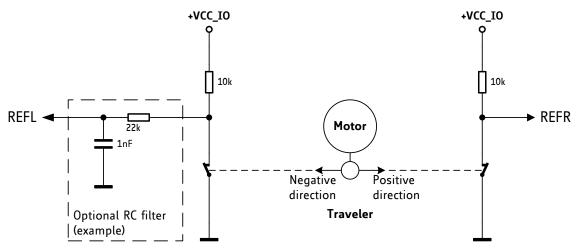
Figure 10.4 Using reference switches (example)
