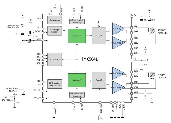
Figure 3.1 Standard application circuit
